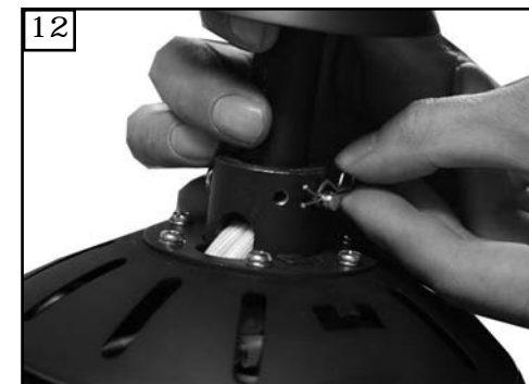
12 Align hole in downrod with hole in yoke and install cross pin. Install downrod into yoke. Install keeper into cross pin.
